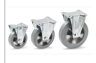
Casings made of steel sheet, galvanized. Wheels with elastic tyres, blue-grey, non-marking (trackless). Alu-rims, hubs with ball bearings. Smooth, silent running, long durability.
