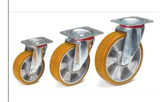
Casings made of steel sheet, galvanized. Wheels with polyurethane tyres, alu-rims, hubs with roller bearings. Smooth, silent running, resisting to many aggressive media, long durability.
