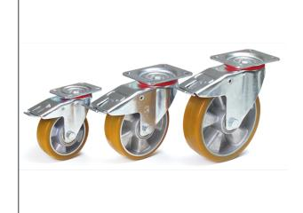
Casings made of steel sheet, galvanized. Wheels with polyurethane tyres, alu-rims, hubs with roller bearings. Smooth, silent running, resisting to many aggressive media, long durability.
