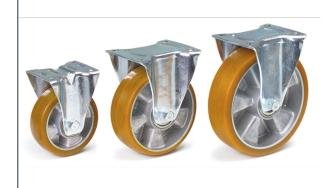
Casings made of steel sheet, galvanized. Wheels with polyurethane tyres, alu-rims, hubs with roller bearings. Smooth, silent running, resisting to many aggressive media, long durability.
