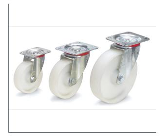
Casings made of steel sheet, galvanized. polyamide wheels, hubs with roller bearings. Largely resisting to humidity, salt, acids and caustic solutions. Temperature-resistant from  $-40^{\circ}$  to  $+90^{\circ}$  C.
