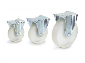
Casings made of steel sheet, galvanized. polyamide wheels, hubs with roller bearings. Largely resisting to humidity, salt, acids and caustic solutions. Temperature-resistant from -40° to  $+90^{\circ}$  C.
