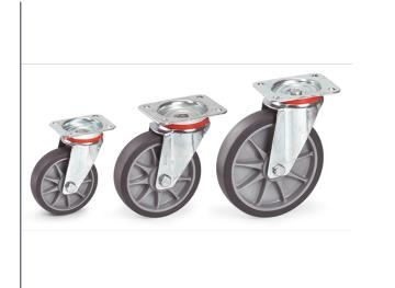
Casings made of steel sheet, galvanized. Plastic rims, hubs with ball bearing and thread protection. Very low starting, rolling and swivelling resistance. Wheels non-marking (trackless).
