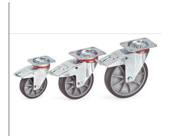
Casings made of steel sheet, galvanized. Plastic rims, hubs with ball bearing and thread protection. Very low starting, rolling and swivelling resistance. Wheels non-marking (trackless).
