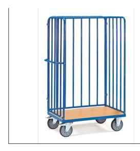
Made of tubular and sectional steel, welded and powder-coated blue RAL 5007, bolted construction. Ends of tubular construction with intermediate uprights at intervals of approx. 130 mm. Detachable side panel. Platform made of special wood material boards, surface beech grain. Wheels: 2 swivel and 2 fixed-wheel castors, TPE tyres, hubs with precision deep grove ball bearing. Swivel castors with wheel locks, according to the European Standard EN 1757-3 (safety of platform trolleys).
