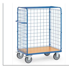
Made of tubular and sectional steel, welded and powder coated blue RAL 5007, bolted construction. Ends and 1 side made of wire lattice 100 x 100 x 5 mm. Platform made of special wood material boards, surface beech grain. Wheels: 2 swivel and 2 fixed-wheel castors, TPE tyres, hubs with precision deep grove ball bearing. Swivel castors with wheel locks, according to the European Standard EN 1757-3 (safety of platform trolleys).
