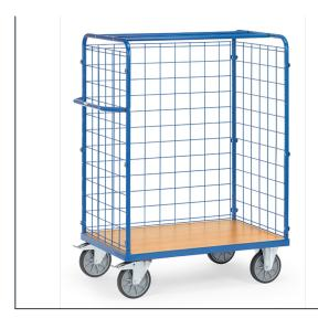
Made of tubular and sectional steel, welded and powder coated blue RAL 5007, bolted construction. Ends and 1 side made of wire lattice 100 x 100 x 5 mm. Platform made of special wood material boards, surface beech grain. Wheels: 2 swivel and 2 fixed-wheel castors, TPE tyres, hubs with precision deep grove ball bearing. Swivel castors with wheel locks, according to the European Standard EN 1757-3 (safety of platform trolleys).
