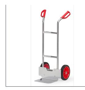
Aluminium trucks made of tubular aluminium with alu blades, very light and handy to use. Aluminum sheet shovel mountable, therefore exchangeable. Curved top bar and transversal struts. For safe transport of circular items such as rolls, cans, buckets etc. Pneumatic tyres on synthetic rims, hubs with roller bearings. Flat packed delivery.
