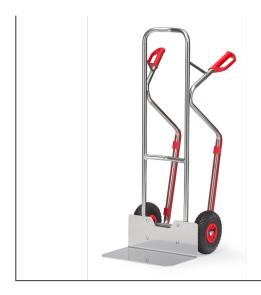
Aluminium trucks made of tubular aluminium with alu blades, very light and handy to use. Aluminum sheet shovel mountable, therefore exchangeable. Curved top bar and transversal struts. For safe transport of circular items such as rolls, cans, buckets etc. Pneumatic tyres on synthetic rims, hubs with roller bearings. Flat packed delivery.
