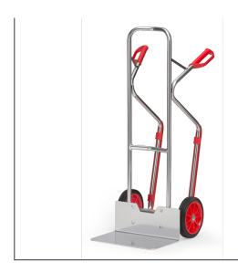
Aluminium trucks made of tubular aluminium with alu blades, very light and handy to use. Aluminum sheet shovel mountable, therefore exchangeable. Curved top bar and transversal struts. For safe transport of circular items such as rolls, cans, buckets etc. Pneumatic tyres on synthetic rims, hubs with roller bearings. Flat packed delivery.
