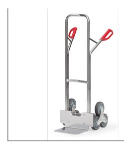
Aluminium tube with aluminium blades, handy welded construction. Safety handles. Aluminum sheet shovel mountable. With 2 three-armed wheel spiders, each equipped with 3 TPE tyres 160 mm Ø. Curved top bar and transversal struts. For safe transport of circular items such as rolls, cans, buckets etc. Flat packed delivery.
