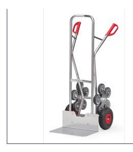
Aluminium tube with aluminium blades, handy welded construction. Safety handles. Aluminum sheet shovel mountable. With 2 pneumatic tyres on synthetic rims, hubs with roller bearings and 2 five-armed wheel spiders, each equipped with 5 TPE wheels 125 mm Ø, hubs with bush bearings. Curved top bar and transversal struts. For safe transport of circular items such as rolls, cans, buckets etc. Flat packed delivery.
