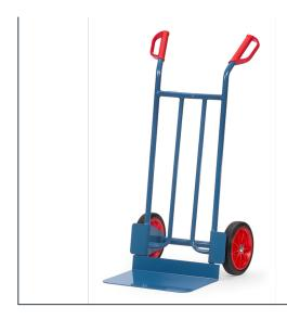
Handy tubular steel trucks with steel sheet blades, sturdy welded construction, blue RAL 5007. Safety grips. Steel sheet front shovel mountable, therefore exchangeable. Solid rubber tyres on synthetic rims, hubs with roller bearings. Flat packed delivery.
