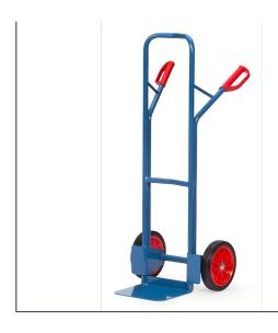
Handy tubular steel trucks with steel sheet blades, sturdy welded construction, blue RAL 5007. Safety grips. Steel sheet front shovel mountable, therefore exchangeable. Solid rubber tyres on synthetic rims, hubs with roller bearings. Curved top bar and transversal struts. For safe transport of circular items such as rolls, cans, buckets etc. Flat packed delivery.
