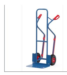
Handy tubular steel trucks with steel sheet blades, sturdy welded construction, blue RAL 5007. Safety grips. Steel sheet front shovel mountable, therefore exchangeable. Pneumatic tyres on synthetic rims, hubs with roller bearings. Curved top bar and transversal struts. For safe transport of circular items such as rolls, cans, buckets etc. Flat packed delivery.
