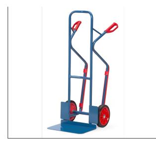
Handy tubular steel trucks with steel sheet blades, sturdy welded construction, blue RAL 5007. Safety grips. Steel sheet front shovel mountable, therefore exchangeable. Solid rubber tyres on synthetic rims, hubs with roller bearings. Curved top bar and transversal struts. For safe transport of circular items such as rolls, cans, buckets etc. Flat packed delivery.
