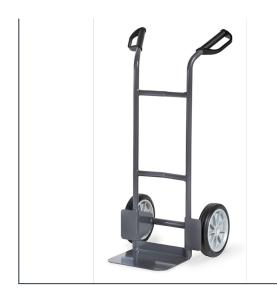
ESD-tubular steel truck with steel sheet blades, sturdy welded construction, electrically conductive powder coating, slate grey RAL 7015. ESD-Safety grips. Steel sheet front shovel screwed on, therefore exchangeable. ESD-solid rubber tyres on synthetic rims, hubs with roller bearings. Curved top bar and transversal struts. For safe transport of circular items such as rolls, cans, buckets etc.
