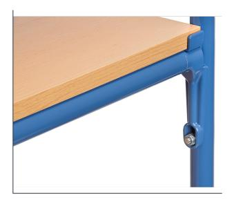
These struts in blue are easily screwed under an existing shelf. That stabilises the upper structure and increases the capacity of the inserted shelves. The shelf located on top of the longitudinal connector struts has a carrying capacity of 150kg instead of 90kg due to the support. 1 pair per trolley is included.
