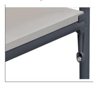
These struts in anthracite grey are easily screwed under an existing shelf. That stabilises the upper structure and increases the capacity of the inserted shelves. The shelf located on top of the longitudinal connector struts has a carrying capacity of 150kg instead of 90kg due to the support. 1 pair per GREY EDITION trolley is included.
