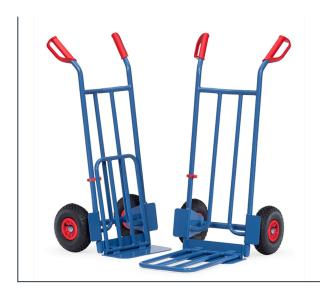
Handy tubular steel trucks with big collapsible lifting blade. Sturdy welded construction, powder coated, blue RAL 5007. Curved top bar and transversal struts. For safe transport of circular items such as rolls, cans, buckets etc. Safety grips, pneumatic tyres on synthetic rims, hubs with roller bearings. Flat packed delivery.
