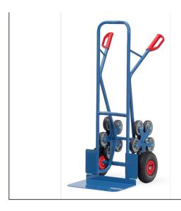
Tubular steel, with lifting blades made of steel plate, sturdy welded construction, powder coated, blue RAL 5007. Safety handles. With 2 pneumatic tyres on synthetic rims, hubs with roller bearings and 2 five-armed wheel spiders, each equipped with 5 TPE wheels 125 mm Ø, hubs with bush bearings. Curved top bar and transversal struts. For safe transport of circular items such as rolls, cans, buckets etc. Steel sheet front shovel mountable. Flat packed delivery.
