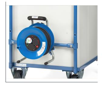
Cable drum as a mounting kit for MultiVario table top carts 500 mm wide. Powder-coated blue RAL 5007. Easy assembly to the support tubes of the carts with clamps. Thermo protected (acc. to VDE) coated cable 3 x 1.5. Lockable with padlock (not included in delivery). For models 2400, 2400B, 2400W, 2420, 2500, 2500B, 2560, 8100, 8200, 8240, 8120, 8220
