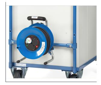
Cable drum holder as a mounting kit for light table top carts 600 mm wide. Powder-coated blue RAL 5007. Easy assembly to the support tubes of the carts with clamps. Thermo protected (acc. to VDE) coated cable 3 x 1.5. Lockable with padlock (not included in delivery). For models 1602, 1802, 2742, 2752, 2942, 2952, 2622, 3742, 3762, 2702, 2722, 2632, 2633, 2634, 2635, 2435, 2436, 2437, 2438, 2105, 2106, 2107, 2108, 4550, 5834, 5836, 5839, 5844, 5837, 5838, 5862, 5864, 5866, 5868
