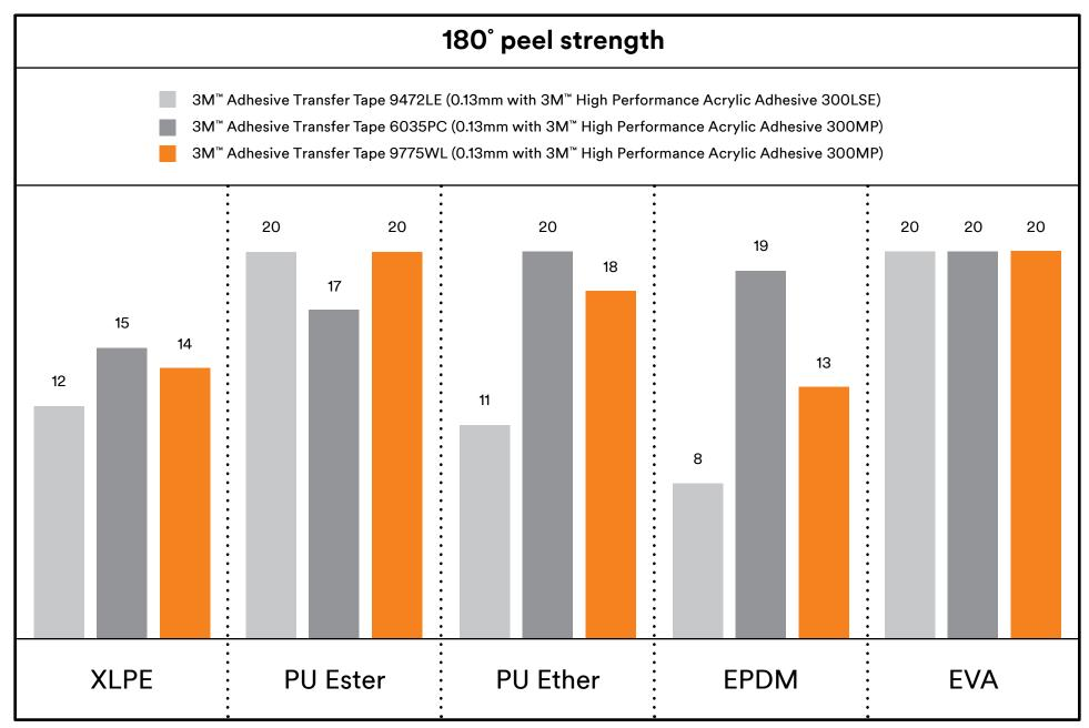
The value of the y-axis is related to the amount of foam tear during the peel procedure. The higher the value, the more foam tear.
