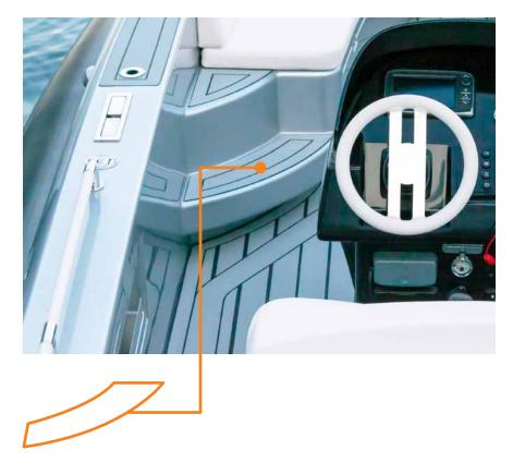
Attach EVA foam boat decking to fiberglass with gelcoat with 3M<sup>™</sup> Adhesive Transfer Tape 9775WL
