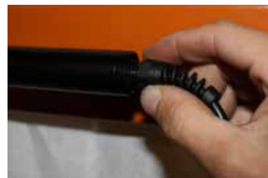
Tighten carefully by hand to make waterproof
