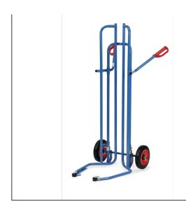
Welded, powder coated, surface durably protected, resistant to impact and scratches. Wheels with solid rubber tyres. Hubs with roller bearings. By activating the hand grips, the truck spreads its carrier spars so that the piles of tyres can be taken up and down directly. The pick up rolls at the tip of the carrier spar support and make the process easier. Suitable for tyres from 450 up to 750 mm Ø. Up to 8 wheels and tyres possible.
