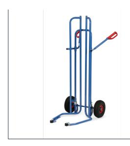
Welded, powder coated, surface durably protected, resistant to impact and scratches. Wheels with pneumatic tyres. Hubs with roller bearings. By activating the hand grips, the truck spreads its carrier spars so that the piles of tyres can be taken up and down directly. The pick up rolls at the tip of the carrier spar support and make the process easier. Suitable for tyres from 450 up to 750 mm Ø. Up to 8 wheels and tyres possible.
