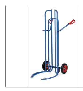
Welded, powder coated, surface durably protected, resistant to impact and scratches. Wheels with solid rubber tyres. Hubs with roller bearings. By activating the hand grips, the truck spreads its carrier spars so that the piles of tyres can be taken up and down directly. Suitable for tyres from 450 to 860 mm Ø. Up to 8 wheels and tyres possible.
