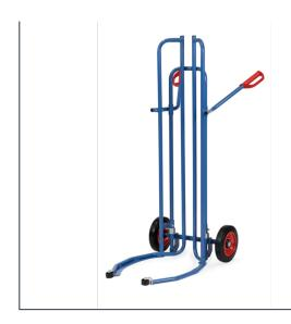
Welded, powder coated, surface durably protected, resistant to impact and scratches. Wheels with solid rubber tyres. Hubs with roller bearings. By activating the hand grips, the truck spreads its carrier spars so that the piles of tyres can be taken up and down directly. The pick up rolls at the tip of the carrier spar support and make the process easier. Suitable for tyres from 450 to 860 mm Ø. Up to 8 wheels and tyres possible.
