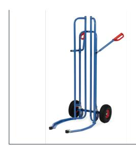
Welded, powder coated, surface durably protected, resistant to impact and scratches. Wheels with pneumatic tyres. Hubs with roller bearings. By activating the hand grips, the truck spreads its carrier spars so that the piles of tyres can be taken up and down directly. The pick up rolls at the tip of the carrier spar support and make the process easier. Suitable for tyres from 450 to 860 mm Ø. Up to 8 wheels and tyres possible.
