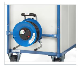
Cable drum as a mounting kit for light table top carts 800 mm wide. Powder-coated blue RAL 5007. Easy assembly to the support tubes of the carts with clamps. Thermo protected (acc. to VDE) coated cable 3 x 1.5. Lockable with padlock (not included in delivery). For models 2746, 2756, 2946, 2956.
