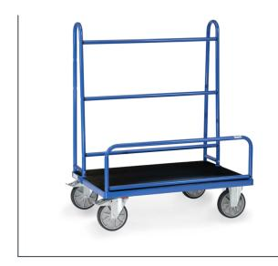
Tubular steel and profile steel welded, powder coated blue RAL 5007. Platform made of derived timber material board, surface covered with corrugated rubber. Bolted tubular steel superstructure. 2 swivel and 2 fixed-wheel castors, TPE tyres, hubs with groove ball bearing. Swivel castors with wheel locks, according to the European Standard EN 1757-3 (safety of platform trolleys). Effective height: 1050 mm, Height retaining bracket: 300 mm.
