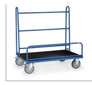
Tubular steel and profile steel welded, powder coated blue RAL 5007. Platform made of derived timber material board, surface covered with corrugated rubber. Bolted tubular steel superstructure. 2 swivel and 2 fixed-wheel castors, TPE tyres, hubs with groove ball bearing. Swivel castors with wheel locks, according to the European Standard EN 1757-3 (safety of platform trolleys). Effective height: 1050 mm, Height retaining bracket: 300 mm.
