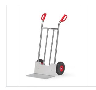
Aluminium trucks made of tubular aluminium with alu blades, very light and handy to use. Aluminum sheet shovel mountable, therefore exchangeable. Punctureproof PU-tyres on synthetic rims, hubs with roller bearings. Flat packed delivery.
