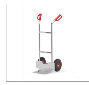
Aluminium trucks made of tubular aluminium with alu blades, very light and handy to use. Aluminum sheet shovel mountable, therefore exchangeable. Curved top bar and transversal struts. For safe transport of circular items such as rolls, cans, buckets etc. Punctureproof PU-tyres on synthetic rims, hubs with roller bearings. Flat packed delivery.
