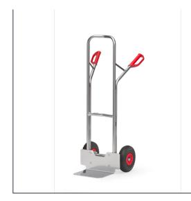
Aluminium trucks made of tubular aluminium with alu blades, very light and handy to use. Aluminum sheet shovel mountable, therefore exchangeable. Curved top bar and transversal struts. For safe transport of circular items such as rolls, cans, buckets etc. Punctureproof PU-tyres on synthetic rims, hubs with roller bearings. Flat packed delivery.
