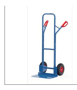
Handy tubular steel trucks with steel sheet blades, sturdy welded construction, blue RAL 5007. Safety grips. Steel sheet front shovel mountable, therefore exchangeable. Punctureproof PU-tyres on synthetic rims, hubs with roller bearings. Curved top bar and transversal struts. For safe transport of circular items such as rolls, cans, buckets etc. Flat packed delivery.
