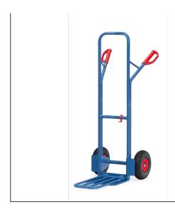
Handy tubular steel trucks with big collapsible lifting blade. Sturdy welded construction, powder coated, blue RAL 5007. Curved top bar and transversal struts. For safe transport of circular items such as rolls, cans, buckets etc. Safety grips, punctureproof PU-tyres on synthetic rims, hubs with roller bearings. Flat packed delivery.
