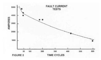
Every cable tested had a single half-lapped layer of 19mm x 0.13mm tinned copper metallic shielding tape for fault current protection. In all cases, the cable's metallic shield was destroyed (by current), whereas, grounding braid remained unharmed.
