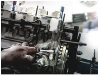
Nutsetter for hexagon head screws
