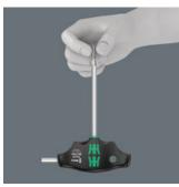
A spring loaded ball ensures the hexagon socket screw to be clamped on the tool tip. Especially helpful in hard to reach areas where you can not use your other hand to hold the screw.
