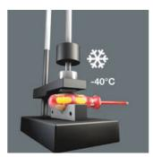
Impact strength tested at -40°C, quaranteeing safety even under extreme conditions.
