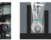
The Joker 6003 ring spanner with its special open end geometry open end offset by 7.5° and the double hexagon profile - doubles the placement possibilities when repeatedly turning the wrench 180° around the longitudinal axis. Bolts and screw heads can be "accessed" every 15°. The Joker 6003 will automatically find the respective placement point after every turn.
