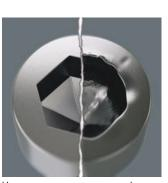
Hexagon screws can endure a problem because the contact surfaces delivering the power from conventional the tool, is transferred to the screw via very small surface areas. The consequence: the screw can become damaged (rounding out). Hex-Plus tools have a greater contact surface that prevents this from happening! At the same time, as much as 20 % more torque can be applied. Good to know: Hex-Plus tools fit into every standard hexagon socket screw!
