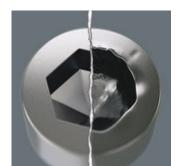
Hexagon screws can endure a problem because the contact surfaces delivering the power from conventional the tool, is transferred to the screw via very small surface areas. The consequence: the screw can become damaged (rounding out). Hex-Plus tools have a greater contact surface that prevents this from happening! At the same time, as much as 20 % more torque can be applied. Good to know: Hex-Plus tools fit into every standard
