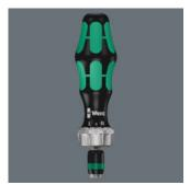
Ratchet screwdriver, fine-tooth design for minimal return angle, switchover ring (right, locked, left), maximum torque of up to 50 Newton metres, 1/4" hexagon chuck with Rapidaptor technology i.e. rapid-in, rapid-out, rapid-spin, chuck-all and single-hand function for rapid bit change, magnetic, suitable for hexagon socket insert bits as per DIN ISO 1173-C 6.3 and E 6.3 and Wera series 1 and 4
